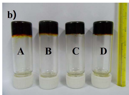
Figure 1. (a) Differential scanning calorimetric (DSC) thermograms for EMI and \text{SiO}_2 NP doped \text{P}_{13}\text{I} electrolytes. (b) Photograph of the solid-state electrolytes A–D at 60^\circ\text{C} .
